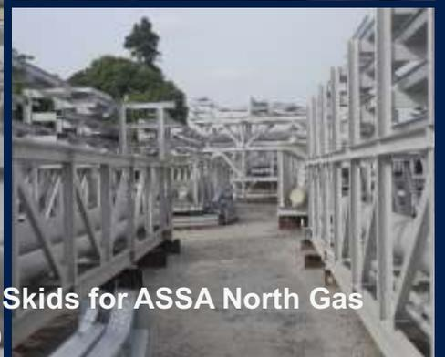
**Fabrication & Assembly of 22nrs of Pipe Racks & Manifold Skids for ASSA North Gas
