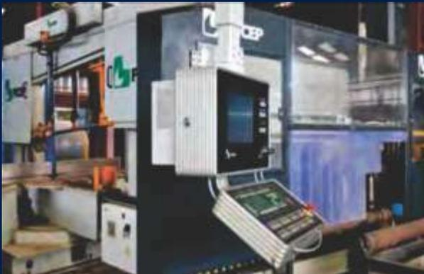
**CNC Controlled Profile Sawing Machine** A multi spindle drilling and sawing line capable of handling a profile of 1000mm width with precision drilling, sawing and beveling capabilities for the fabrication of structural steel with zero errors and human intervention
