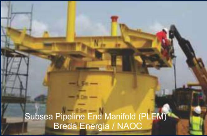
Subsea Pipeline End Manifold (PLEM)
